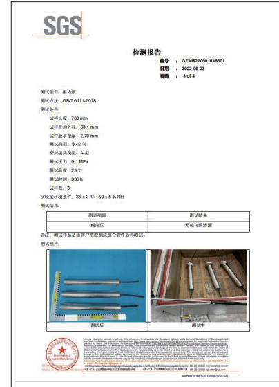
Water resistant pressure 0.1MPa test report of foam
