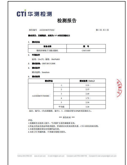
Compressive strength 2.26MPa test report of foam
